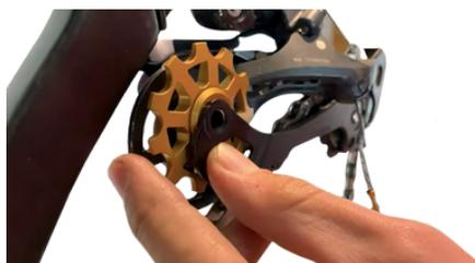
**Replace the Shimano pulley by a Nova pulley.**
