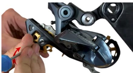
**Screw the pulley back on with the same screw.**
