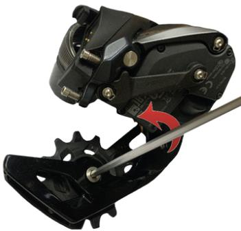
**Remove the second SRAM pulley by using the 5mm allen key.**
