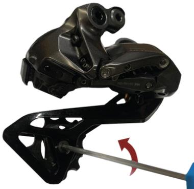
**Unscrew the second pulley by using the 5mm Allen key.**
