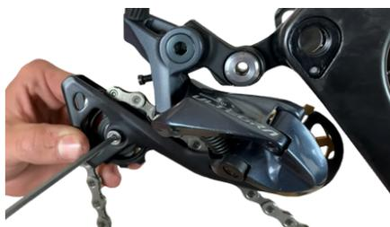
**Remove the second Shimano pulley by using the 5mm Allen key.**
