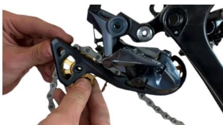
**Replace the second Shimano pulley with the Nova pulley.**
