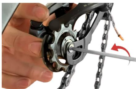
**First remove the pulley using a 5mm (Shimano) or a 4mm (SRAM) Allen key.**
